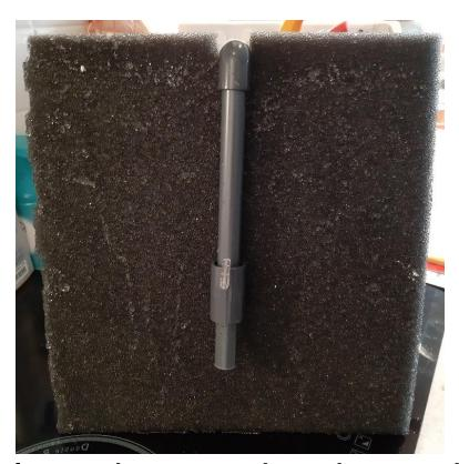
lower inlet. This is a chamber with top and bottom sealing rings and the uplift tube has tiny holes drilled through so a foam of air, rather than bubbles, gathers and lifts water up the tube. Hence it was silent too.
