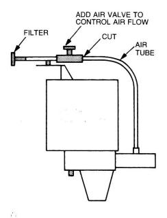
If you use a power filter with built-in aeration you may get too much air – to reduce this means slowing the pump down and so reduced filtration.
