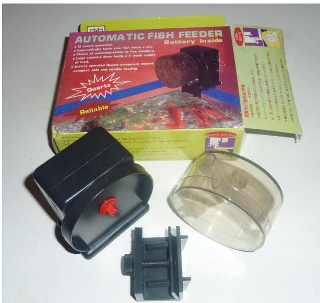
The 'included' battery is inserted and the red axle turns slowly through 360 degrees in 24 hours via a clock mechanism (it ticks). The plastic dish fits over this drive, and, when filled with flake or granules, scoops a portion into a chute that allows the feed to fall into the aquarium.
