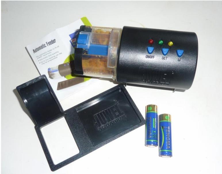
One good example for the single aquarium is the Juwel Autofeeder. The price should be under £25. It is powered by two AA batteries and contains a microchip operated by pressing three buttons. These are for ON/OFF and to select one feed or two feeds every 24 hours....
